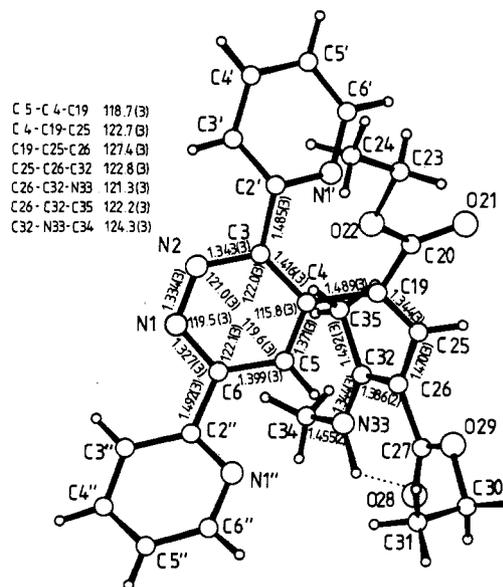
Figure 1. X-ray molecular diagram of compound 5a with crystallographic atomic numbering. Selected bond lengths and bond angles are given (esd's in parentheses).
