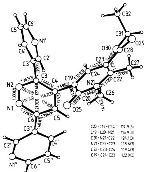
**Figure 2.** X-ray molecular diagram of compound **6b** with crystallographic atomic numbering. Selected bond lengths and bond angles are given (esd's in parentheses).
